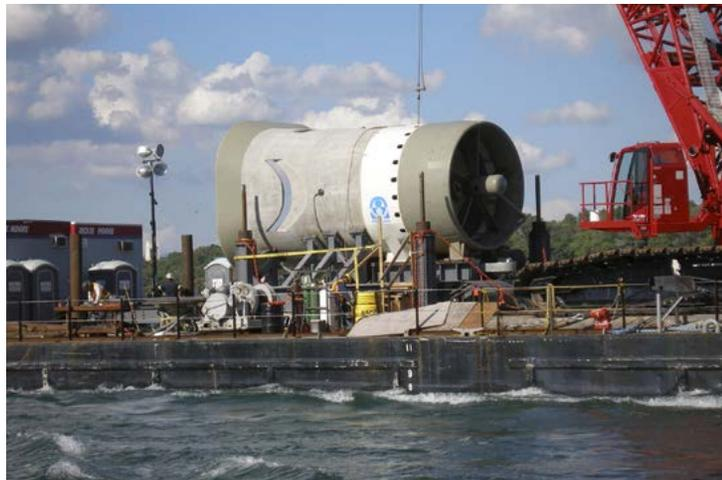
Cover: Model of a horizontal-axis hydrokinetic turbine
