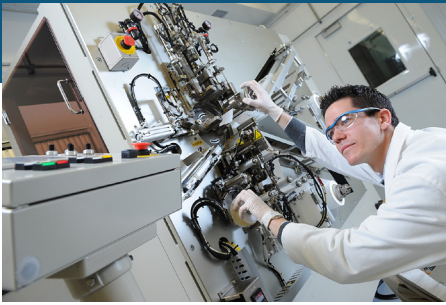
In the dry room, a technician operates a winding machine
