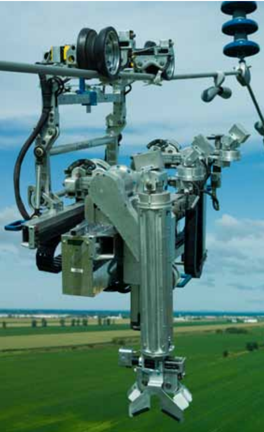
LineScout and its robotic arm
