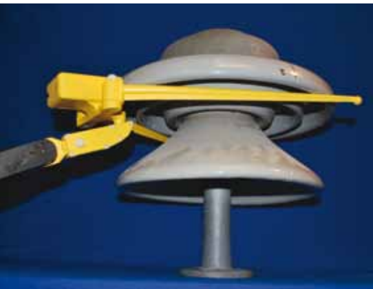
CIAP feelers probing the shed of a 120-kV insulator
