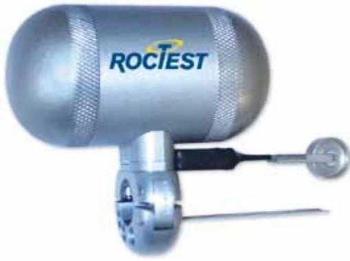
Strain gauges produce a signal proportional to the dynamic bending amplitude of the conductor or ground wire. Pavica measures the signal frequency and amplitude of each vibration cycle and records the data at the desired rate in a counter matrix.
